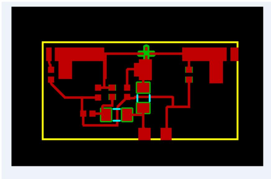
Figure 16: Adjusted Bit Map Layout for Etching
