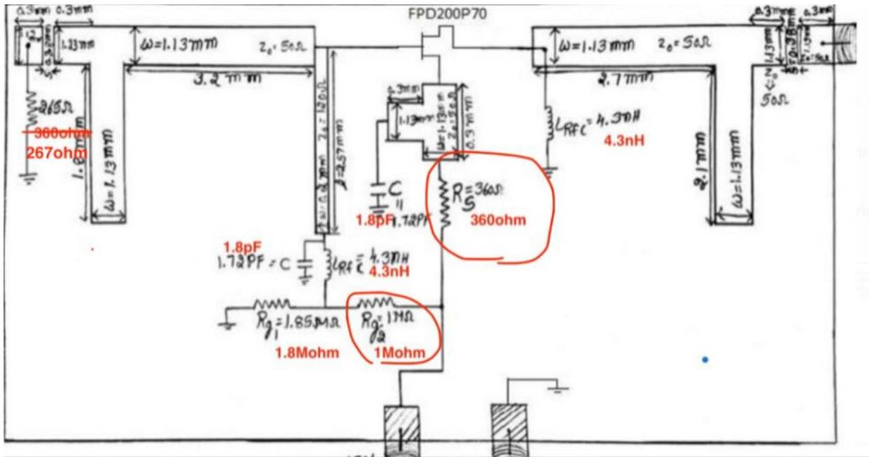
Figure 14: Adjusted component values of the designed circuit.
