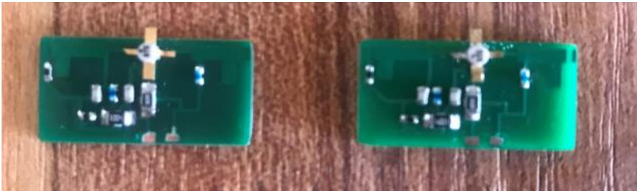
Plate 4: Fabricated oscillators on .8mm and 1.6mm Fr4 substrates
