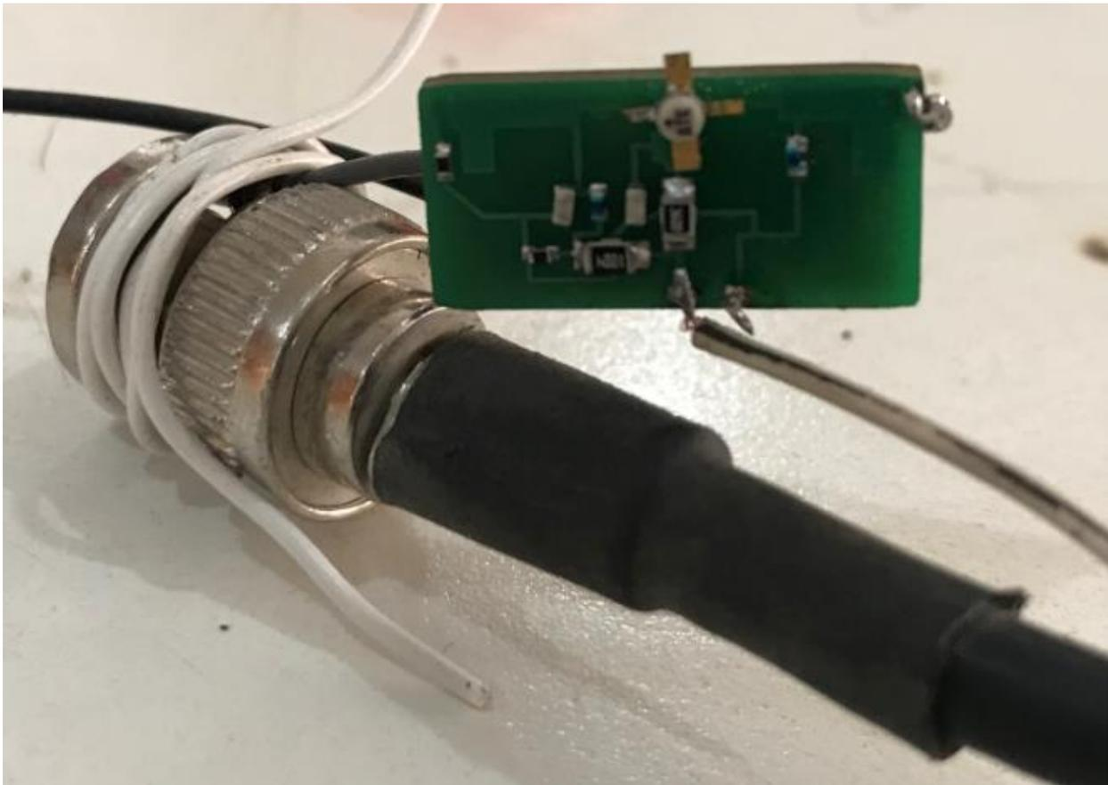
Plate A1, Oscillator circuit connection on Test Rig
