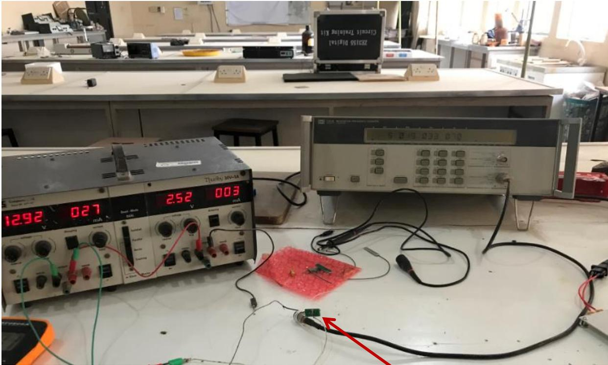
Plate 5: Rig for Testing the Oscillator.
