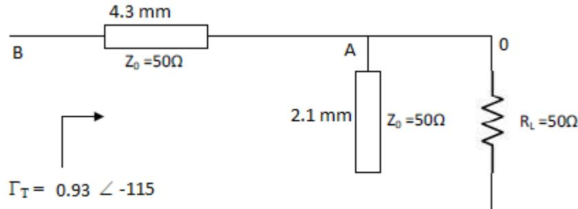
Figure10: Circuit for terminating network
