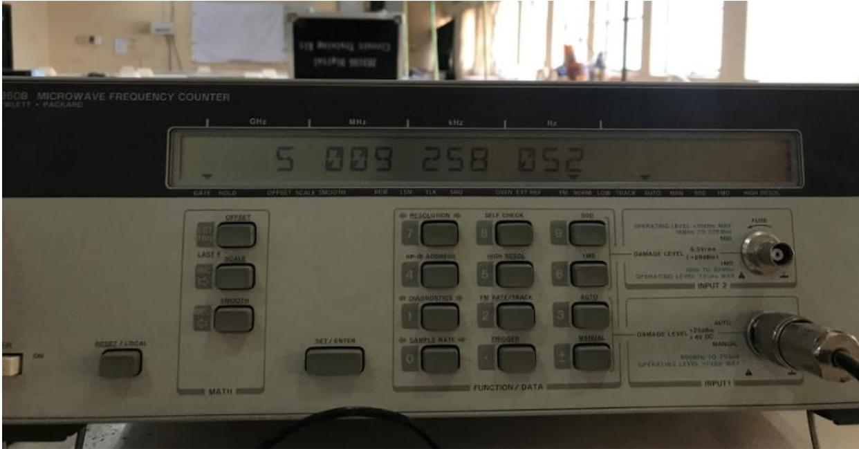
Plate 6: Frequency generated by the Oscillator
