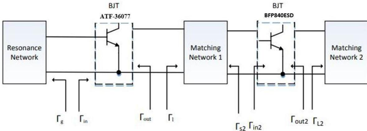
Figure 1: Oscillator with One stage Amplification
