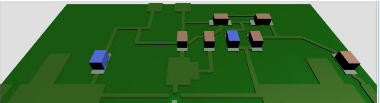
Figure 18: Inverted Proteus 3D layout of Oscillator Circuit
