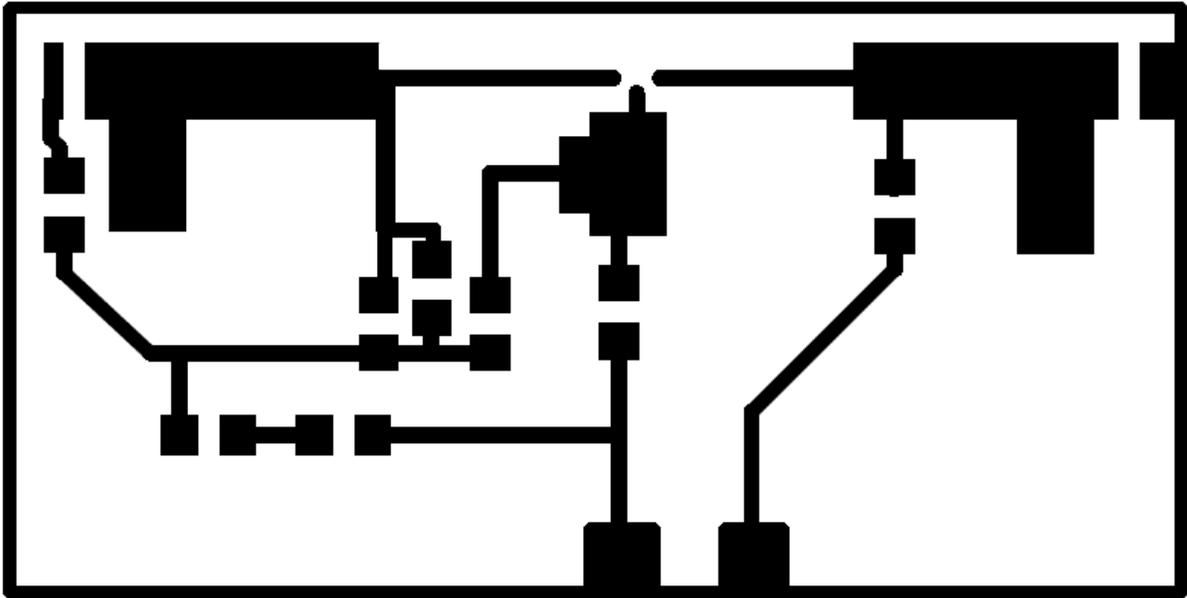
Figure 15: Circuit layout for Etching PDF
