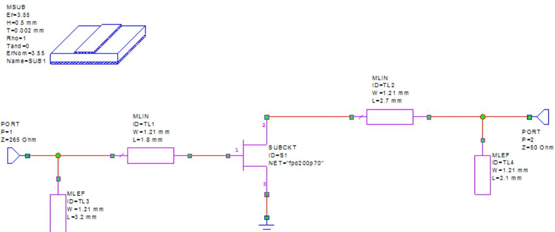
Figure 11: Transmission line circuit for Generator tuning and Terminating Network
