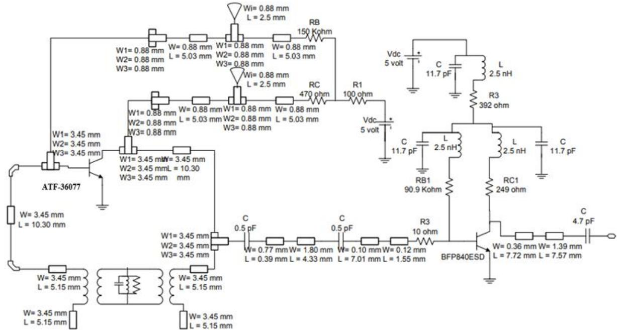
Figure 2: Circuit Diagram of the oscillator 1 in ADS platform
