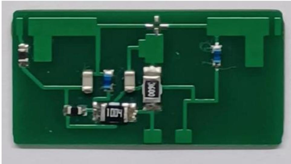
Plate 3: Fabricated oscillator layout on Fr4 substrate
