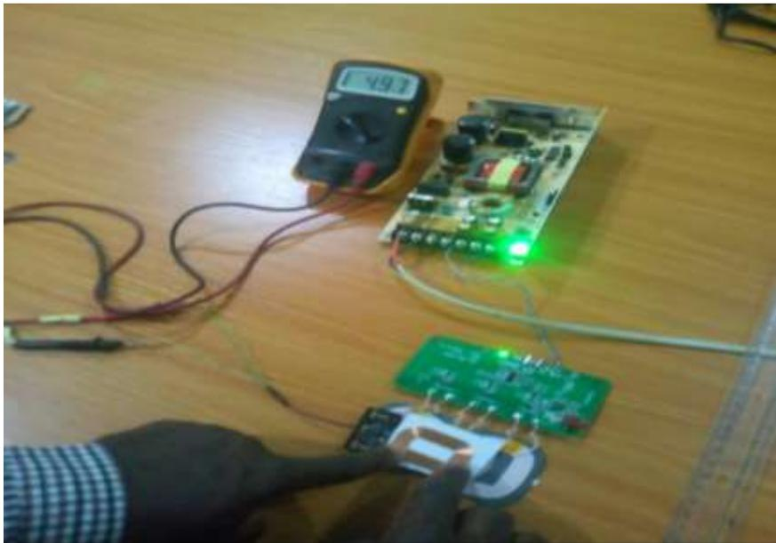
Fig 47: Measurement of the Receiver voltage at 2mm lift off.
