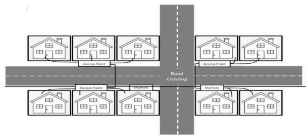
Figure 15: Dual side duct
