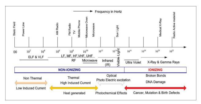
**Figure 1: Electromagnetic Field Range**
