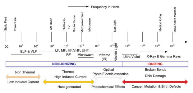
Figure 3: Electromagnetic spectrum
