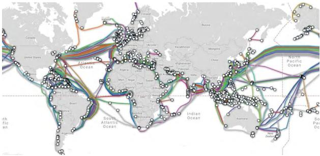
Fig 2.9: World Deep-Sea Backbone connection Source: FCC
