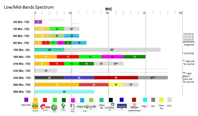
Figure 7.1.1: Assignment of High Demand Spectrum in Nigeria 2020 Source: NCC
