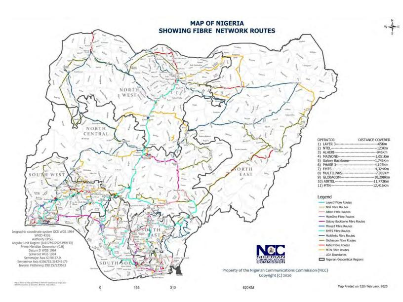
Fig 2.10: Map of Nigeria Fibre Network Routes Q4, 2019 Source: NCC Map is based on data submitted by Network Operators as at Q4, 2019 with exception of Suburban, BCN and 21st Century
