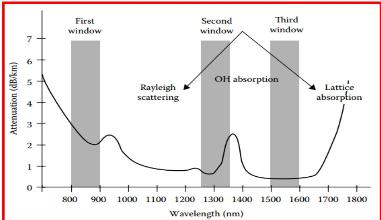
Figure 2.8: Optical Fibre Transmission Windows (Binh, 2015)
