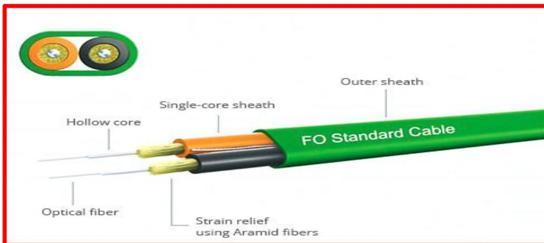
Figure 1.2: Glass Optical Fibre(FONP/FS.com, 2017)
