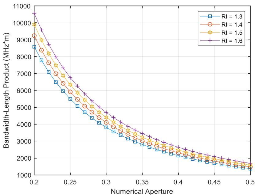
Figure 4.2: Bandwidth-Length Product versus NA
