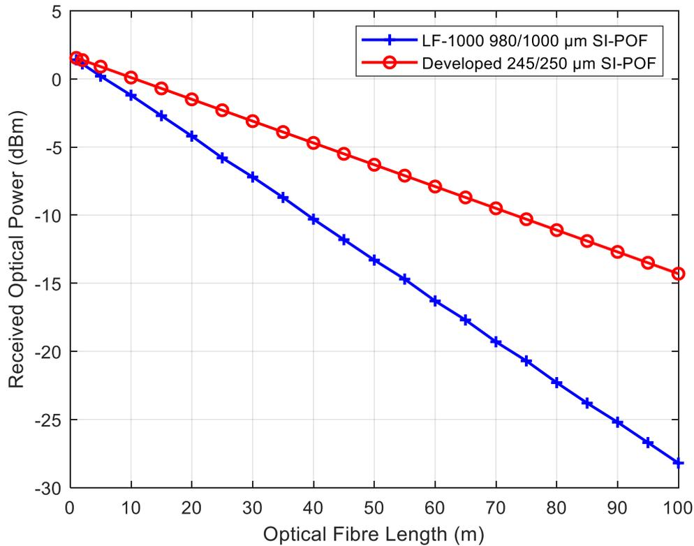
Figure 4.7: Optical Power against Optical Fibre Length
