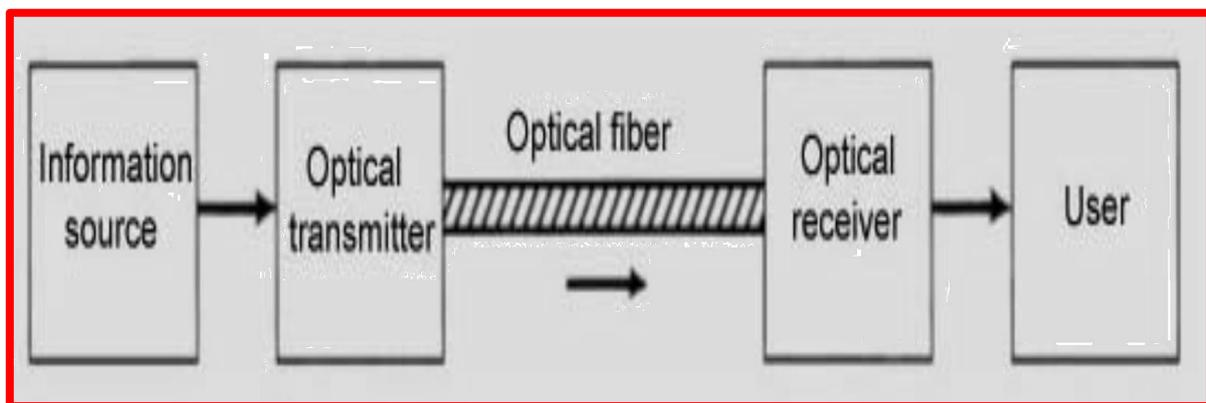
Figure 2.11: A simple point-to-point Optical Fibre Link
