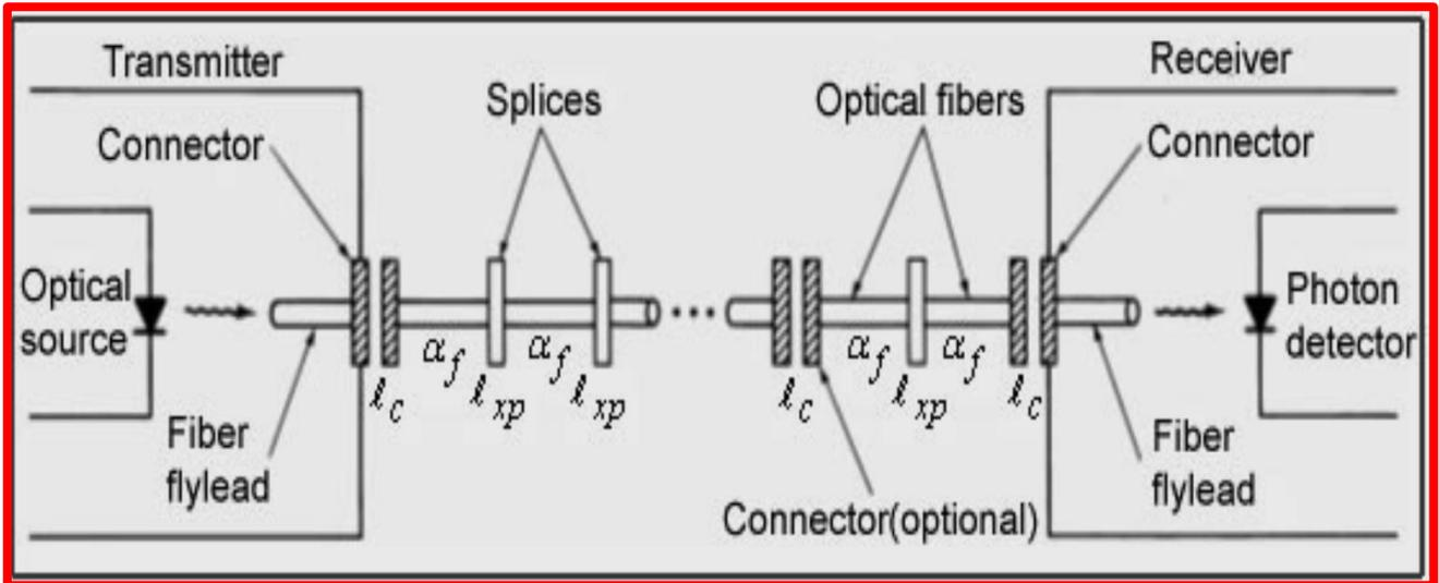
Figure 2.12: Power Loss Model
