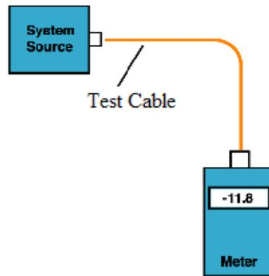
Figure 5: Optical Power Loss Measurement
