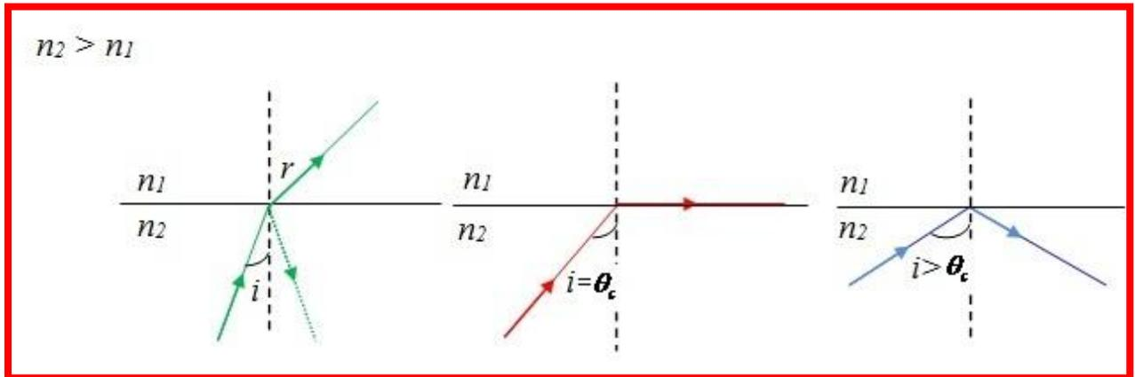
Figure 2.1: Total Internal Reflection (Nelkon and Parker 1995)
