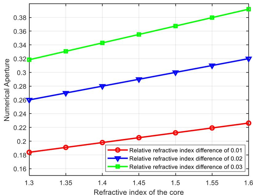
Figure 4.1: NA versus RI of the Core at Different RRI Difference Values
