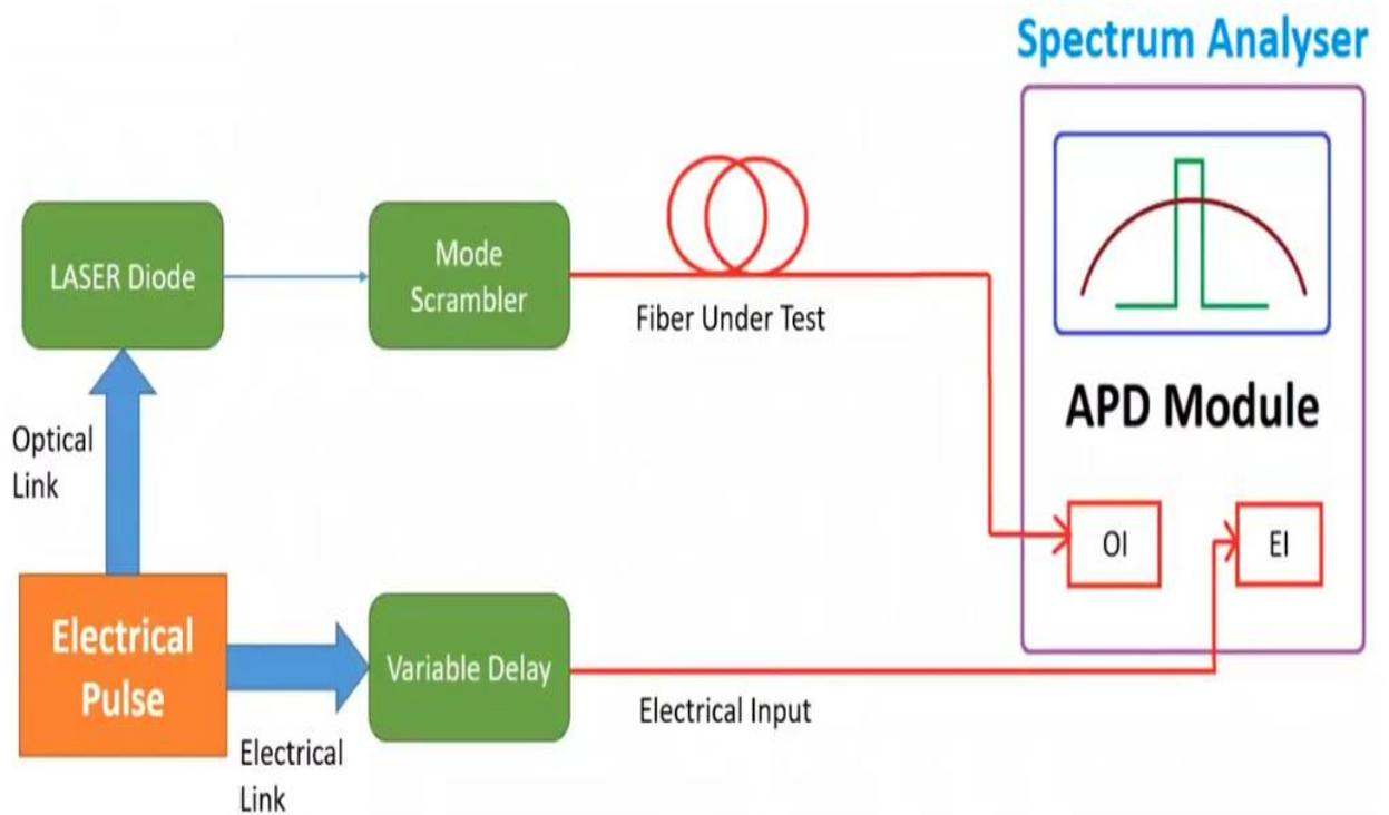
Figure 4: Frequency Domain Measurement of Intermodal Dispersion
