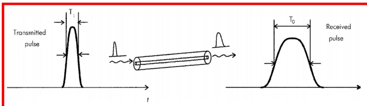
Figure 2.10: Dispersion in Optical Fibre (Zubia and Arrue, 2001)
