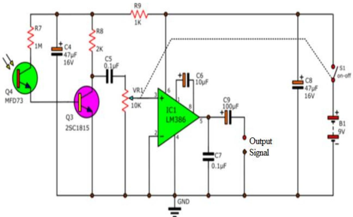
Figure 8: Optical Receiver Circuit
