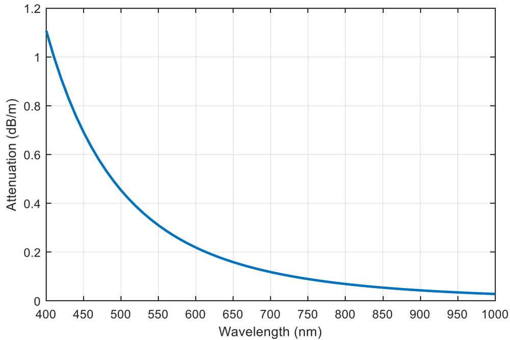
Figure 4.6: Attenuation of the Developed POF against Wavelength
