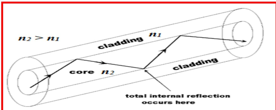
Figure 2.3: Light Propagation along Optical Fibre Cable
