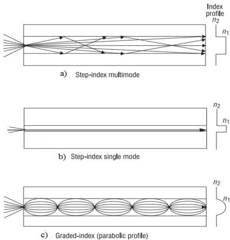
Figure 2.6: Fibre Optic Configurations (Massa, 2000)
