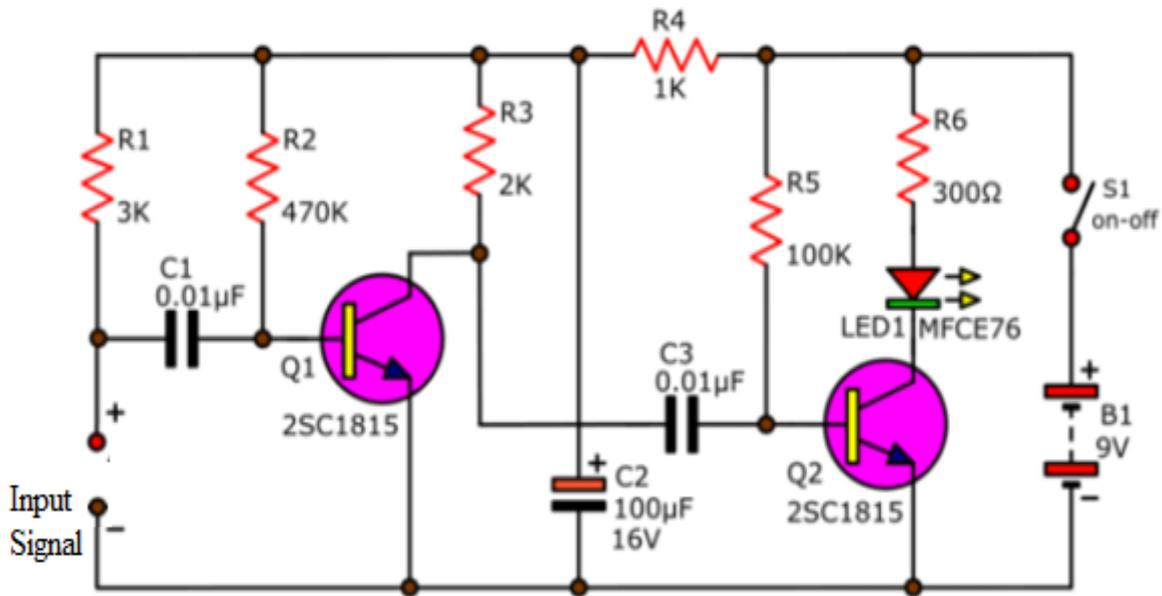
Figure 7: Optical Transmitter Circuit
