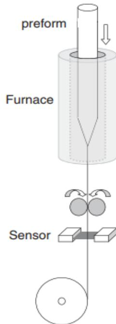
Figure 1: Preform-Drawing Process
