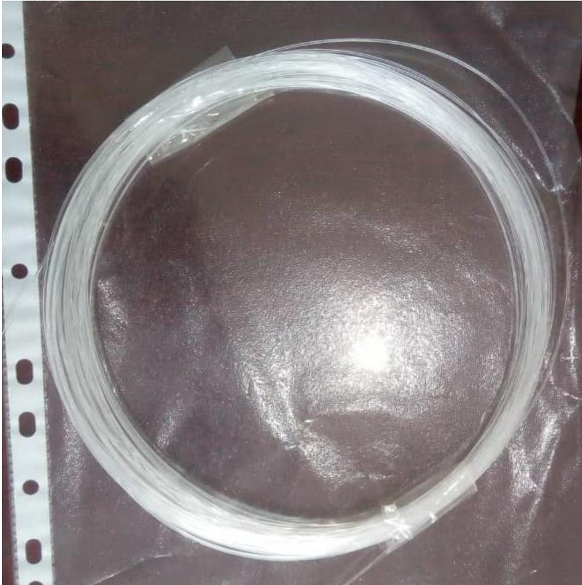
Plate 2: Locally Fabricated 490/500  $\mu\text{m}$  SI-POF
