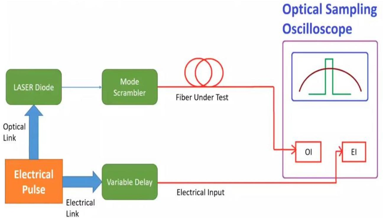
Figure 3: Time Domain Measurement of Intermodal Dispersion
