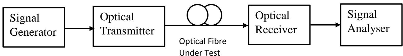
Figure 6: Attenuation Measurement
