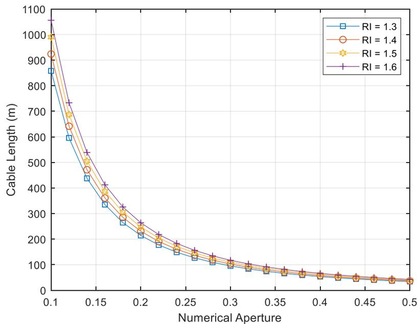
Figure 4.3: Optical Fibre Cable length versus NA at Bandwidth of 40 MHz
