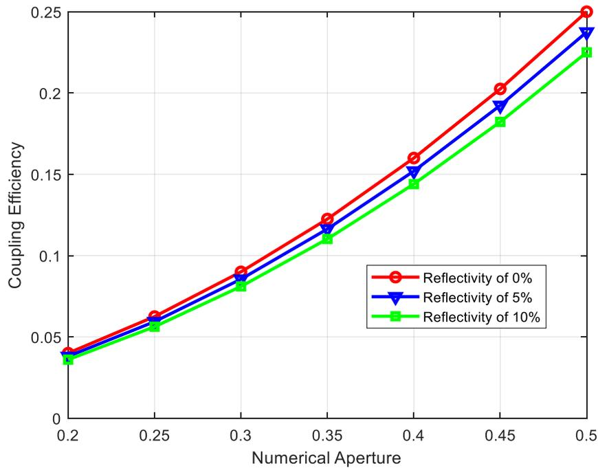
Figure 4.5: Coupling Efficiency versus NA
