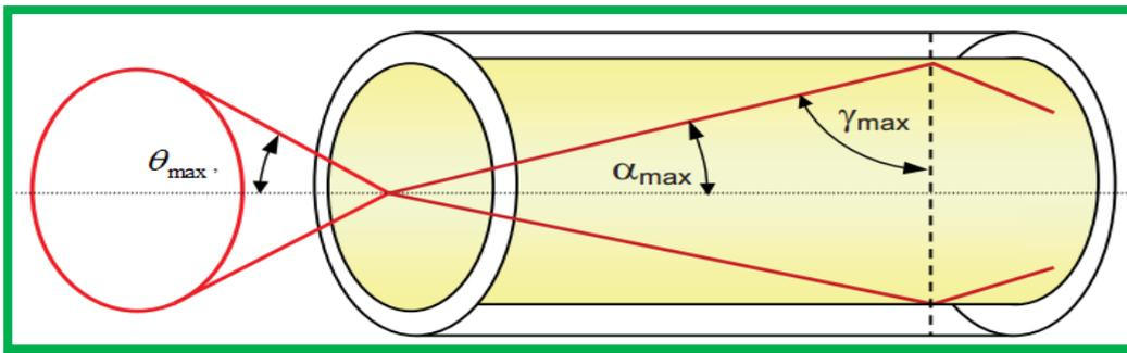
Figure 2.2: Acceptance Angle (Ziemann *et al.*, 2008)
