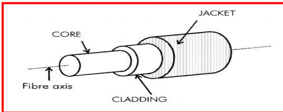
Figure 2.7: Structure of Optical Fibre Cable (Zubia and Arrue, 2001)
