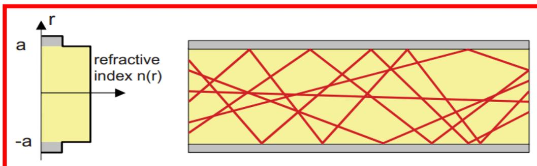
Figure 2.4: Index Profile in Step Index Fibre (Ziemann *et al.*, 2008)
