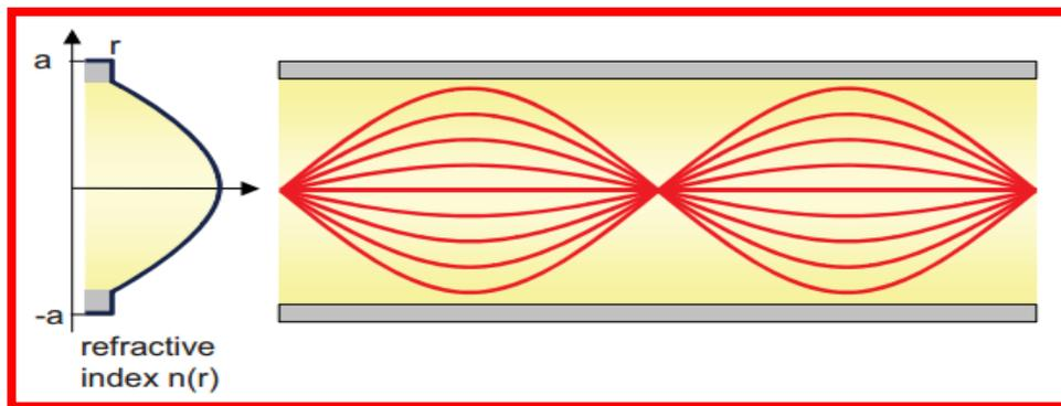
Figure 2.5: Index Profile in Graded Fibre
