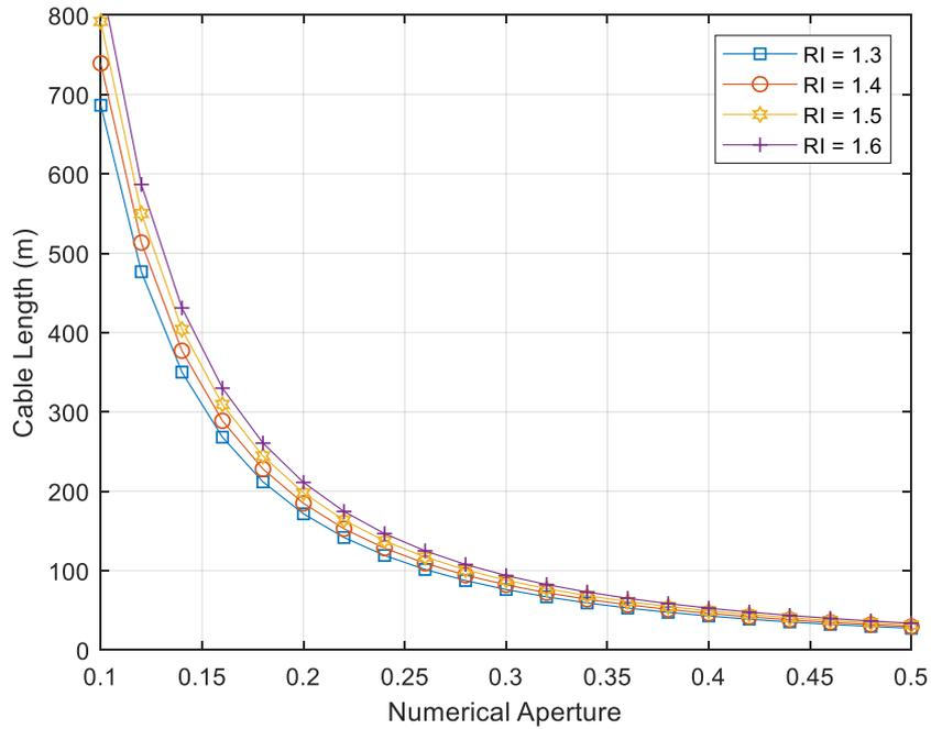
Figure 4.4: Optical Fibre Cable length versus NA at Bandwidth of 50 MHz
