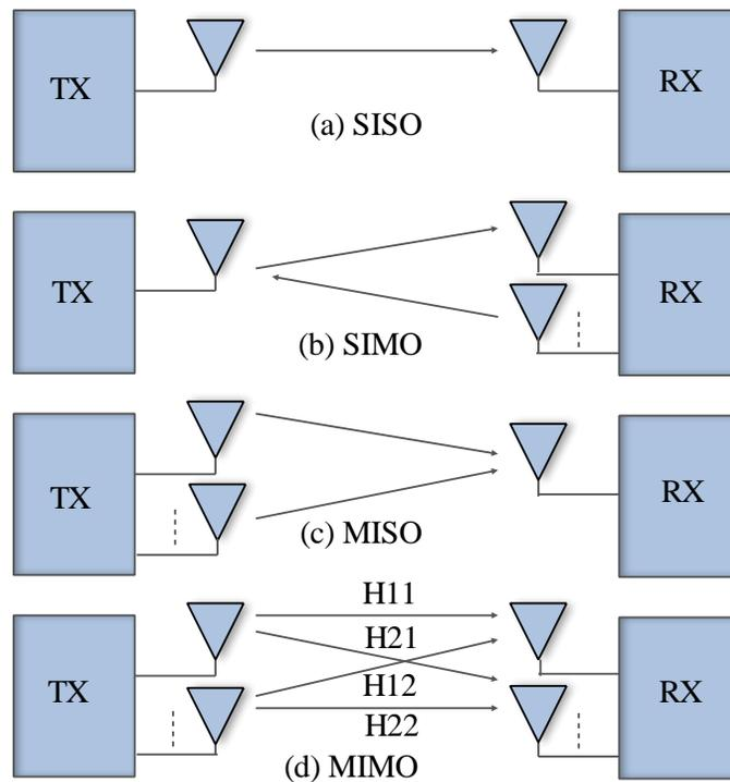
Figure 3.2 Various types of wireless communication.
